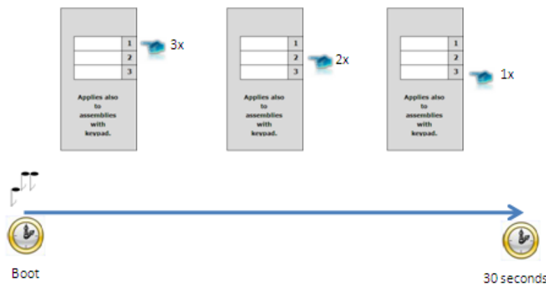
Figure 3.1 Switching to static IP address
